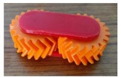
Helical gear mechanisms
