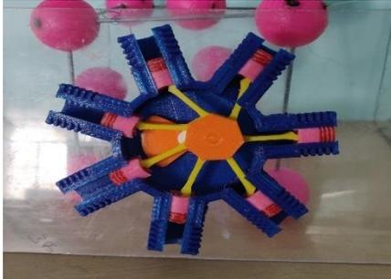
Radial engine Sun and Planet gearing mechanism
