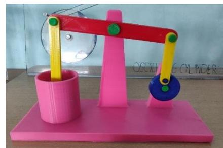
Beam engine mechanism
